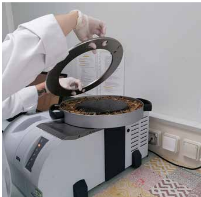
NIRS provides a rapid and accurate analysis of the nutritional value of raw materials and finished products to result in optimum feed formulation.
